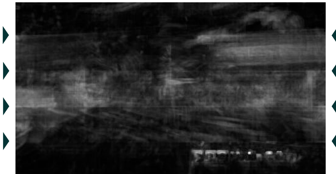
Figure 29: Accumulated SSIM error map of the error propagation processes from 100 randomly selected skipped and replaced slices. For each of those 100 slices individually, the entire BBC video would be compared to the undegraded original. This results in an SSIM error map for each frame, which were added up to the picture shown here. White represents the maximum error, black an error of zero. Therefore, dark areas were generally less affected by errors than bright areas. The arrows to the left and right mark the slice boundaries, which are faintly visible in the image.
