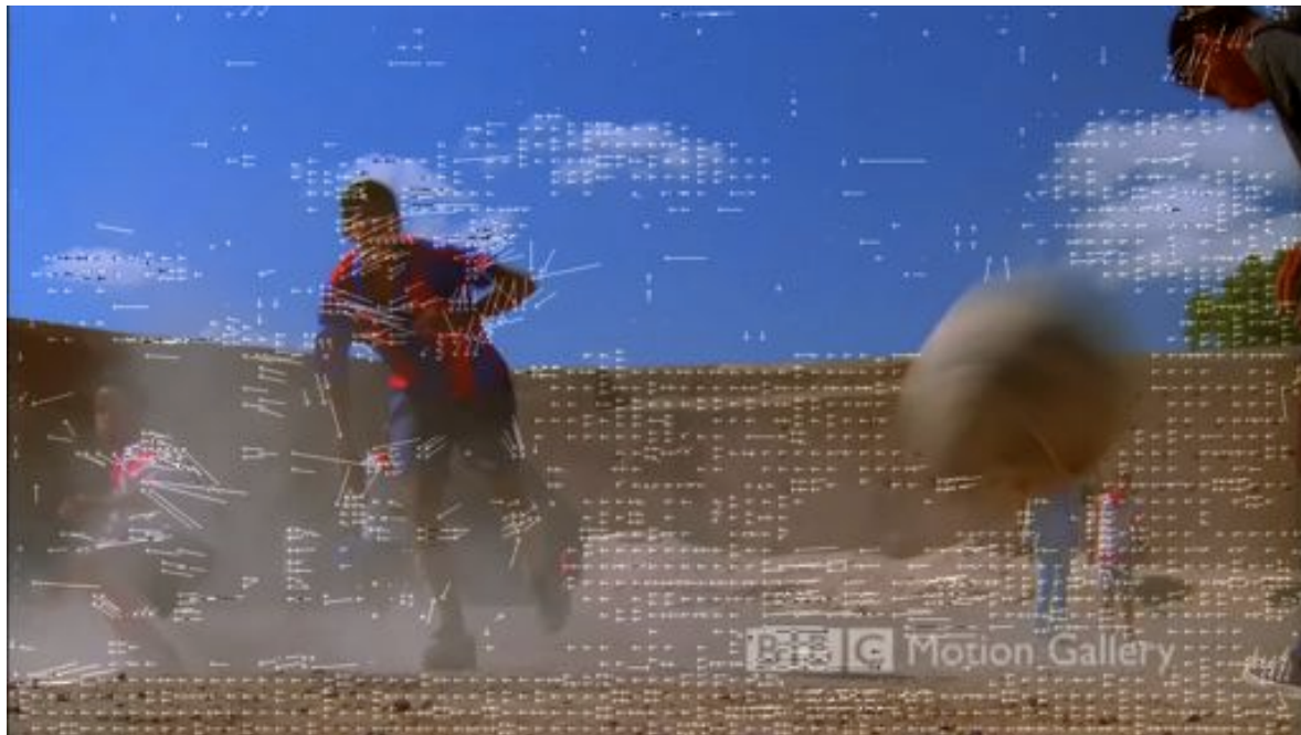
Figure 16: Frame from BBC video with visualized motion vectors as an example for motion blur leading to intra compression. The ball on the right is moving fast toward the camera and will exit the frame on the right edge. Notice that although it is a moving object, no motion vectors encode that motion. Instead, the ball is fully intracoded.
