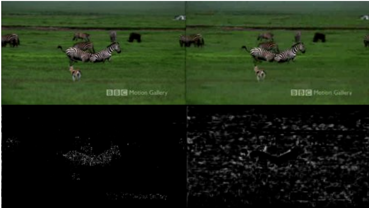
Figure 4: Comparison of MSE and SSIM; upper left: original video frame (from BBC video, see Table 1 on page 18); upper right: video frame degraded by compression artifacts (re-encoded original at 384 kbit MPEG-4 Part 2); lower left: map of Y' component MSE values (black represents 0, white represents 50^{-1} or larger); lower right: map of Y' component local SSIM values (black represents 1, white represents 0). It is clearly visible that SSIM detects the structural loss in the grass regions much better than MSE, which in turn penalizes errors in the zebras that are less disturbing to the viewer.
